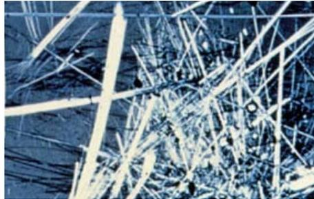
**Figure 4** Asbestos fibres viewed down a microscope
